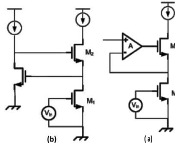
Figure 3: The main idea of Gain Boosting technique, (a) the block diagram, (b) circuit structure [10]
