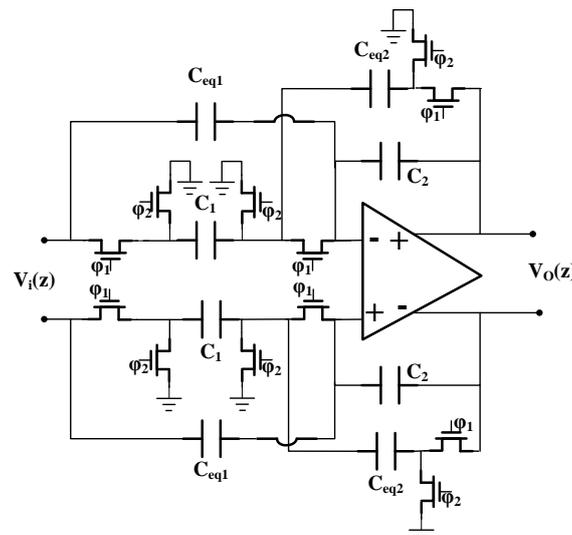
Figure 5: Differential first-order high-pass filter [11] and a sampling frequency of 100 MHz. According to Niquist criterion, the input signal frequency is considered to be less than half the sampling frequency, i.e. less than 50 MHz [11].
