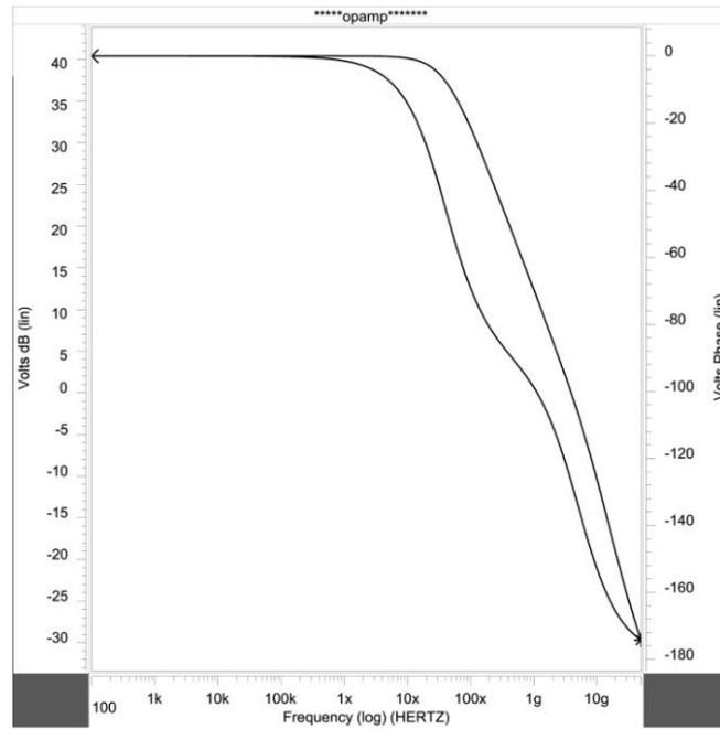
**Figure 6:** Frequency response of the folded Cascode amplifier
