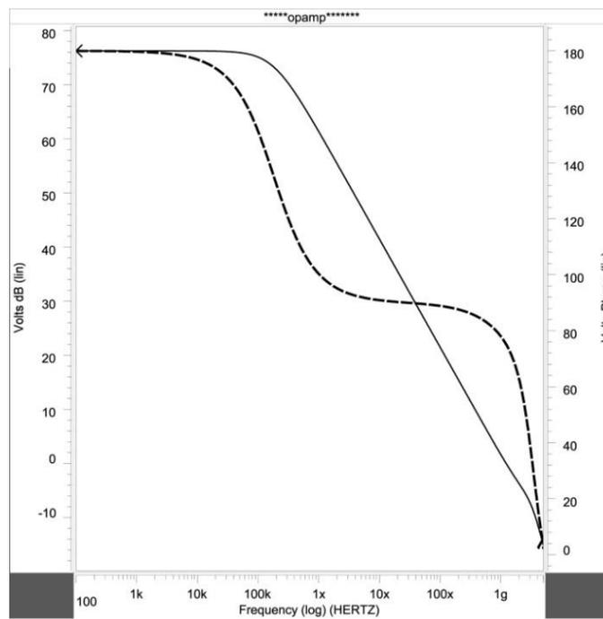
**Figure 7:** Frequency response of the proposed amplifier
