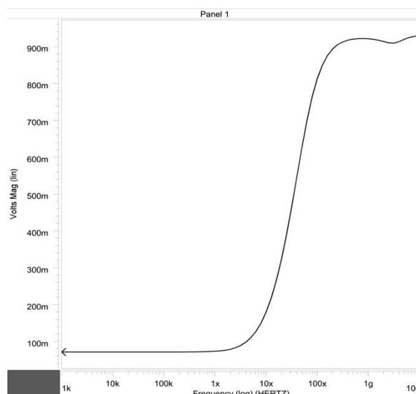
Figure 9: Output of high-pass filter designed with the proposed amplifier
