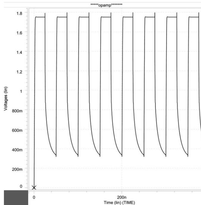
Figure 8: Amplifier response to step input
